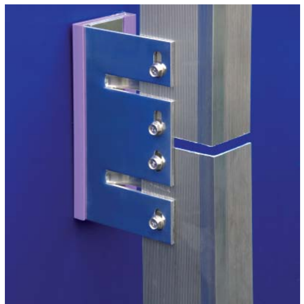
If your Project Checklist Return shows rails joined with a double bracket, a 10mm gap MUST be left between the rails Panels must never span rail joints.
